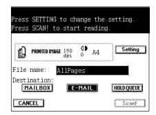
Press the area \_\_\_\_\_as shown on the right to switch to the e-mail address input screen.
